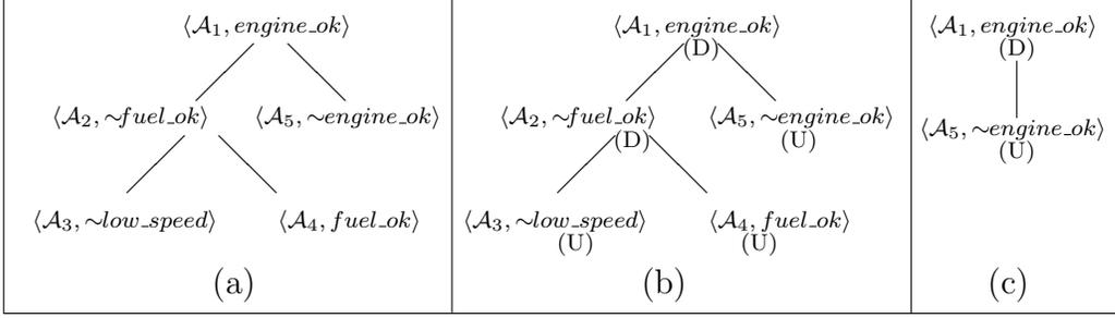
Fig. 2. (a) Dialectical tree for  $\langle \mathcal{A}_1, engine\_ok \rangle$ ; (b) marked dialectical tree for  $\langle \mathcal{A}_1, engine\_ok \rangle$ ; (c) associated pruned dialectical tree
