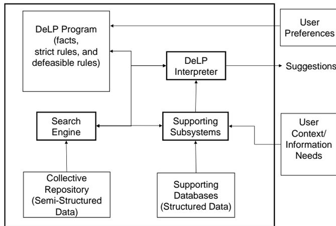
Fig. 3. Argument-Based User Support System based on DeLP
