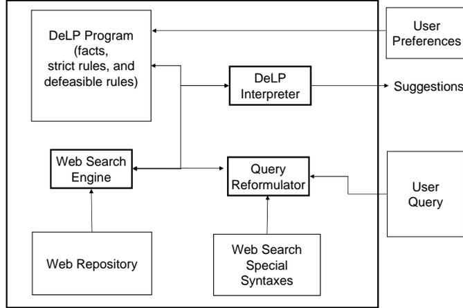
Fig. 4. Argument-Based Web Recommender System based on DeLP
