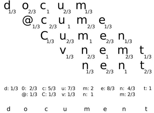
Figure 4: An example of correcting a text with 5-grams and the *triangle* weighting function. The number under every character in the top part is the weight of that character in its position for every window. The mid-bottom table shows the sum of the weights for every candidate character on each position of the output. To generate the final output (at the bottom), the candidate character with the maximum sum on every position is selected.
